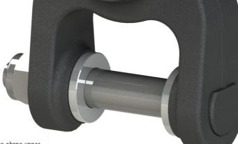
Formiko link FHL 01 is compatible with eye shape upper interface rotators. Various models for rotator upper interface widths 60mm, 73mm, 45mm, rotator and link connecting pin diameter options: 25mm, 30mm,
